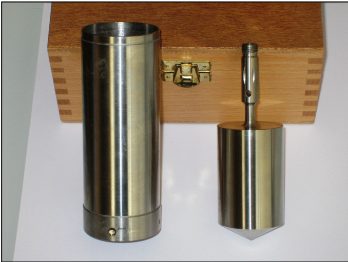
Fig. 1: Coaxial cylinder measuring system, left outer cylinder, right inner cylinder
