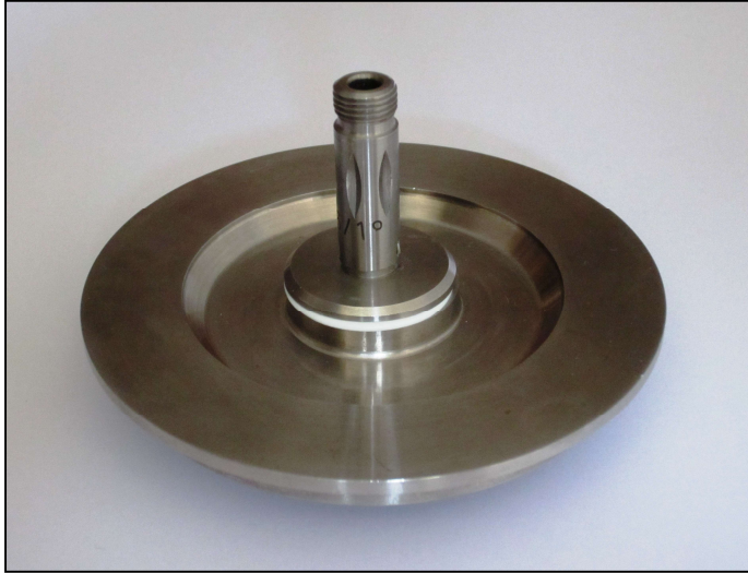
Fig. 2: Cone-plate measuring system, cone angle 1^\circ
