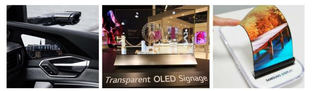
**Figure 2.** OLED applications: replacement of the side-view mirror by an OLED display (left, copyright: Audi AG),<sup>[19]</sup> transparent display (center, copyright: LG Display),<sup>[15]</sup> flexible display (right, copyright: Samsung).<sup>[16]</sup>
