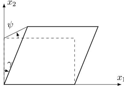
Figure 1.1: Deformation in a simple shear test
