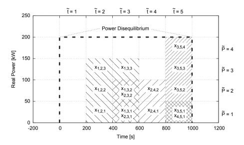
Figure 7.2: An example of a power balance state after the discretization
