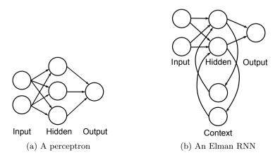
Figure 2.10: Two types of Artificial Neural Networks
