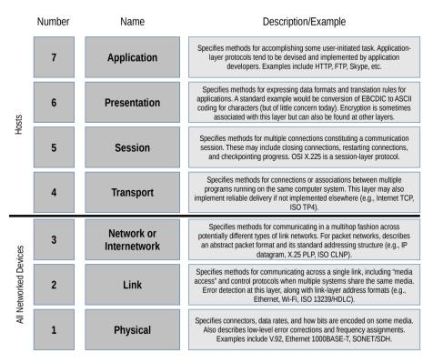
Figure 2.8: The ISO/OSI reference model
