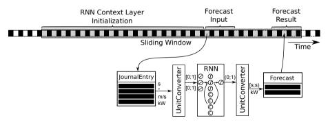
Figure 5.2: The sliding window structure maintained in the forecaster module
