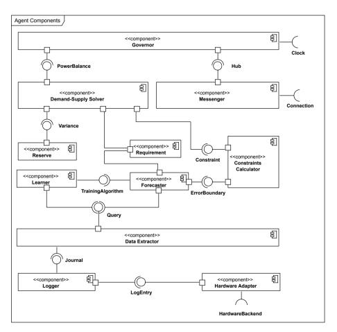
Figure 4.2: Components of the Universal Smart Grid Agent
