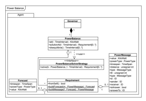
Figure 7.1: The Universal Smart Grid Agent's internal power balance
