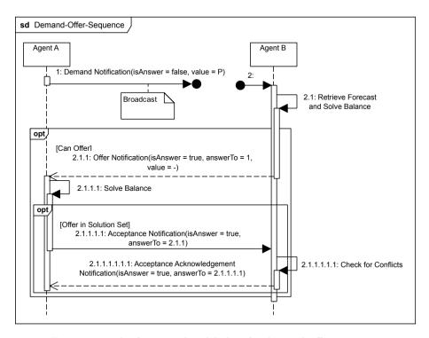
Figure 6.2: The four-way handshake of a demand-offer sequence
