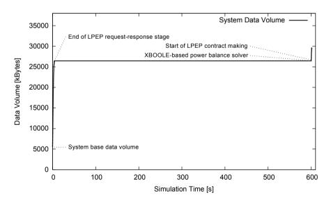
Figure 7.7: Total data volume by time required by the Universal Smart Grid Agent in the Fukui-TEPCO power grid during high load
